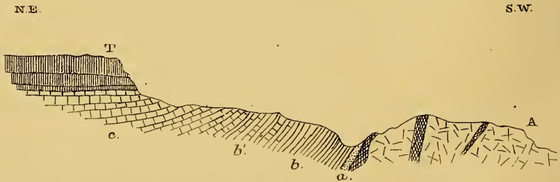
Section through Allur hill :—T. Deccan trap. c. Limestone. b. Calcareous shales, b', Purple shales. a. Basement grit. A. Gneiss, &c.
