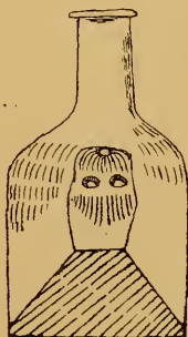
Native smelting furnace used in Sáwant Wári.
